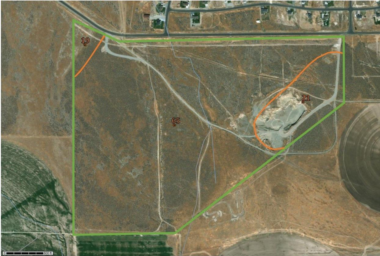
Figure 2. Map of site boundary (green) and different soil units (orange) within the property. Numbers correlate with Table 1.
